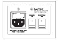
Fig. 2.16: Voltage supply and fuse
